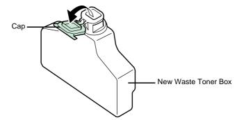
6 Insert the new waste toner box as shown in the figure below. When the box is set correctly, it will snap into place.
